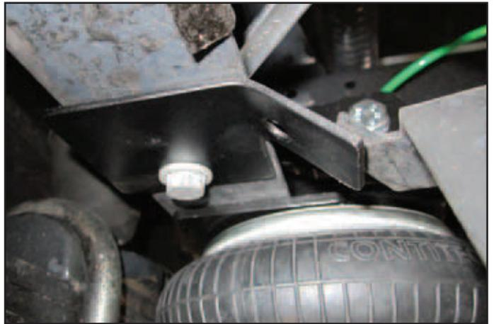
14. Mount the original brake line bracket to the mounted brake line bracket.
