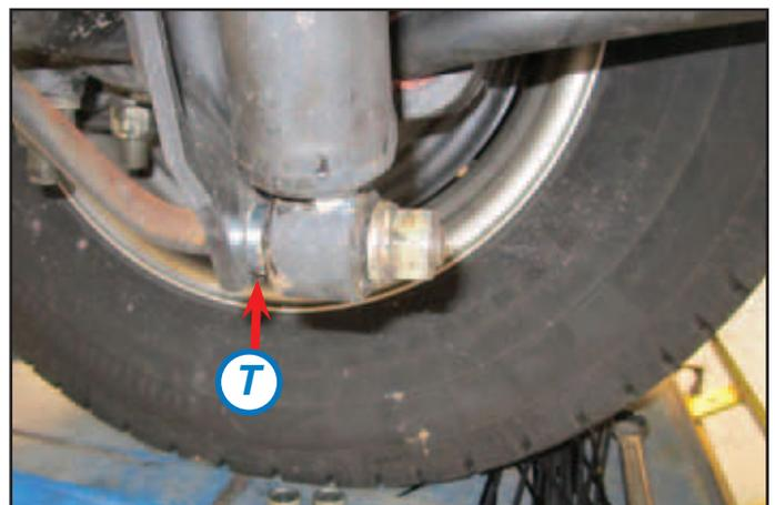
12. Remove the brake line bracket.
